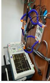
**Figure 1.** Acquisition setup made of a Tektronix H10 H-Field Probe connected to a Tektronix MDO4024C oscilloscope.
